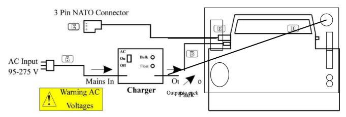
Set the unit to 24V mode and with a suitable voltmeter check the voltages at the points shown.
