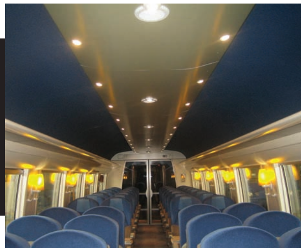
ZTER train, centre ceiling with triple LED down lights.
